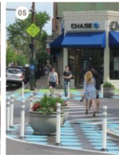
視線引導設施 delineator posts
