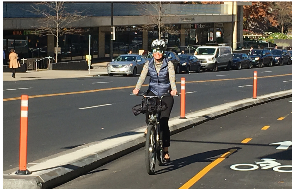
Protected bicycle lane on Staniford Street, Boston
